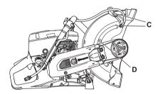
The cutting head is now loose and can be removed from the machine. Remove the belt from the belt pulley.
